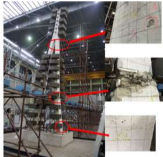
Fig.4 The damage characteristics of the bridge model
