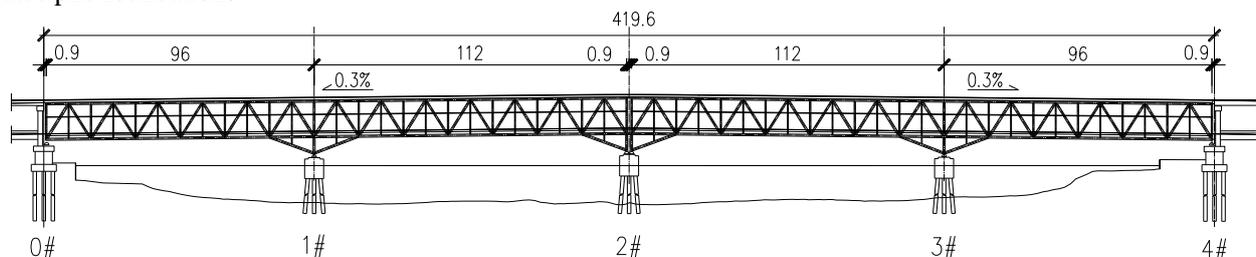
Fig.1 Elevation of the Main Bridge of the Songpu Bridge
