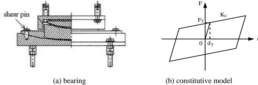
Fig.4 Friction Pendulum Seismic Isolation Bearing
