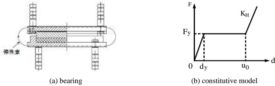
Fig.5 Cable-sliding Friction Aseismic Bearing
