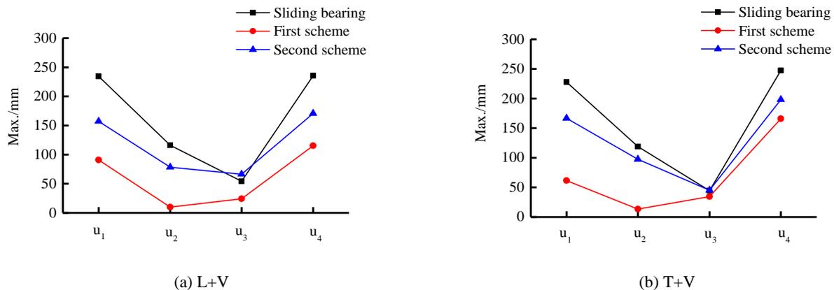
(u<sub>1</sub>: Bearing deformation; u<sub>2</sub>: Residual deformation of the bearing; u<sub>3</sub>: Relative displacement between the adjacent bridge span; u<sub>4</sub>: Relative displacement between the main bridge and the approach bridge)
