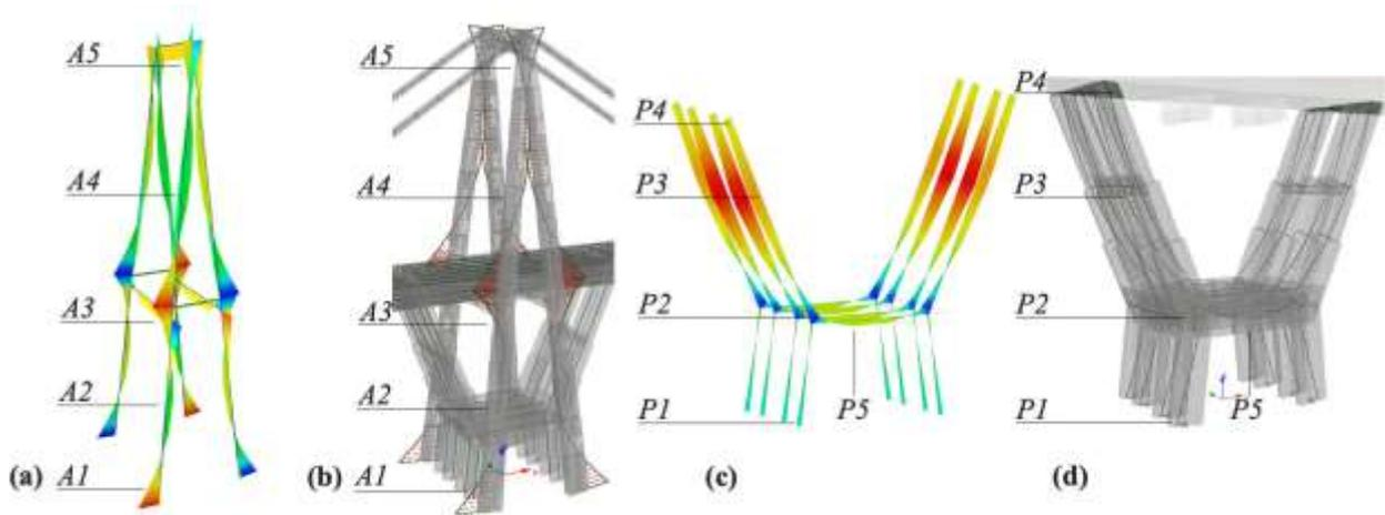
Fig. 4 – (a) Midas Civil Antenna bending moment, (b) SeismoStruct Antenna bending moment, (c) Midas Civil Pier bending moment, (d) SeismoStruct Pier bending moment
