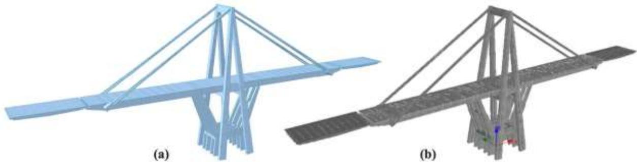
Fig. 3 – Balanced system number 9: (a) Midas Civil, (b) SeismoStruct
