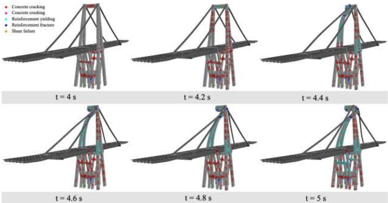
Fig. 12 – Possible collapse scenario triggered by shear failure
