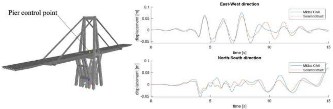
Fig. 7 – Pier displacements comparison
