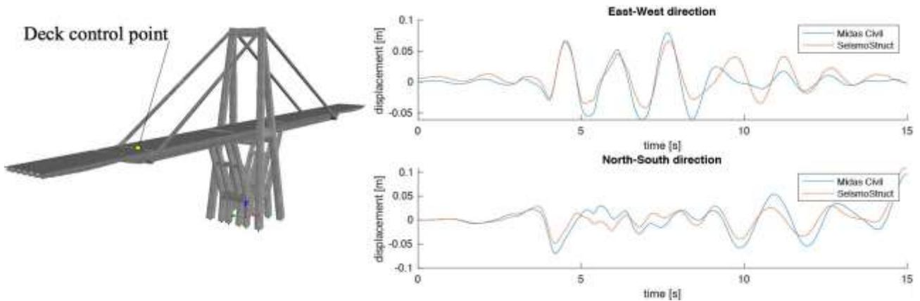
Fig. 8 – Deck displacements comparison
