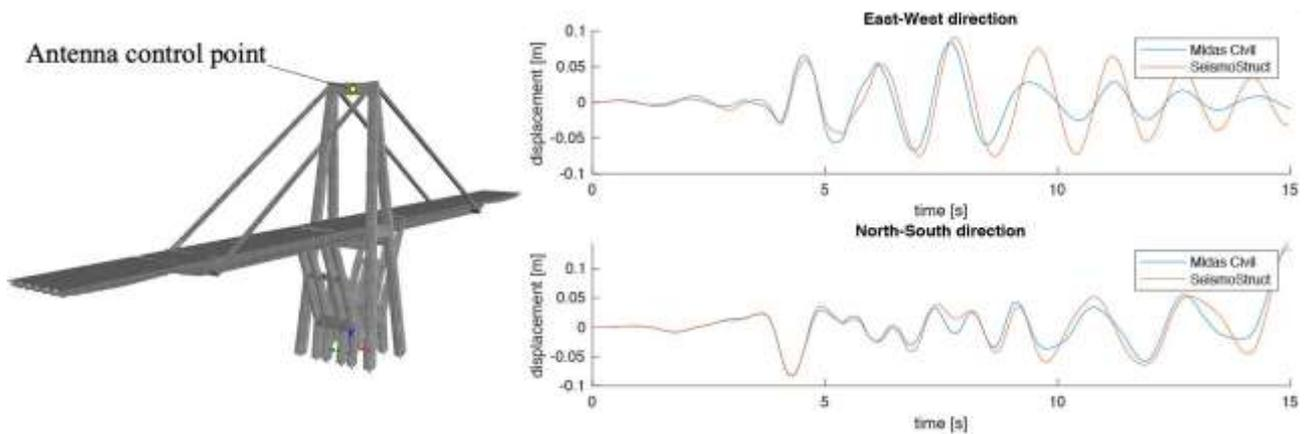
Fig. 6 – Antenna displacements comparison
