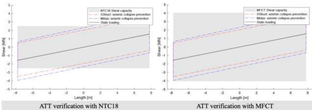
Fig. 11 – Comparison between NTC18 equation and MFCT shear capacity
