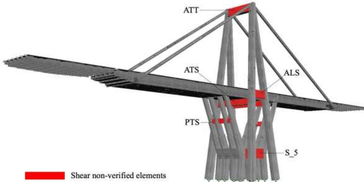
Fig. 10 – Shear non-verified elements
