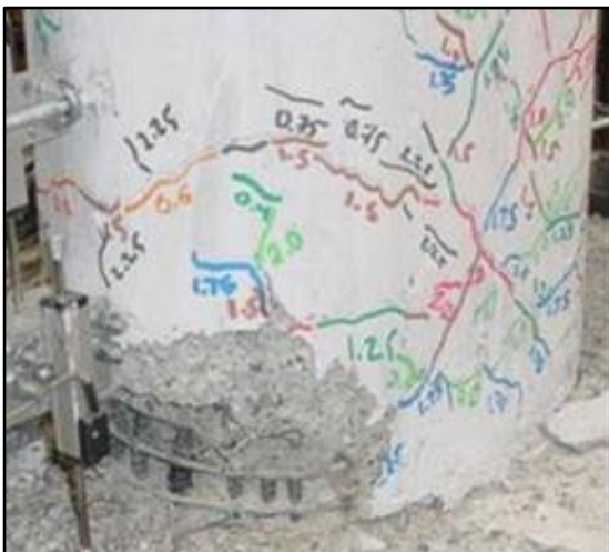
Figure 9 DS-5 Imminent Failure
