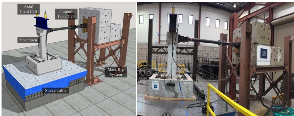
Fig. 2 – Shake table test setup at UNR
