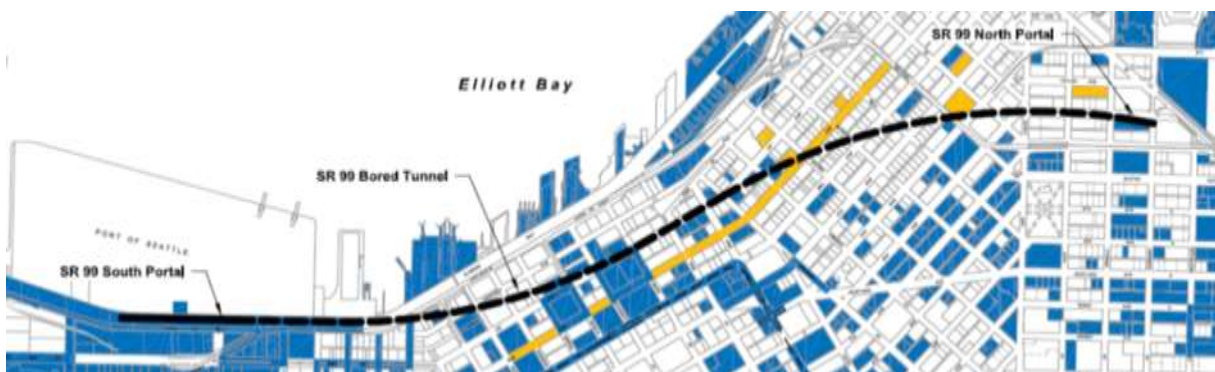
Fig. 1 – SR 99 Tunnel alignment
