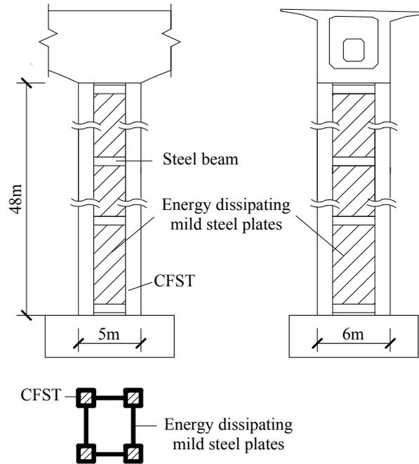
Fig.1 – Concept of innovative pier with composite section
