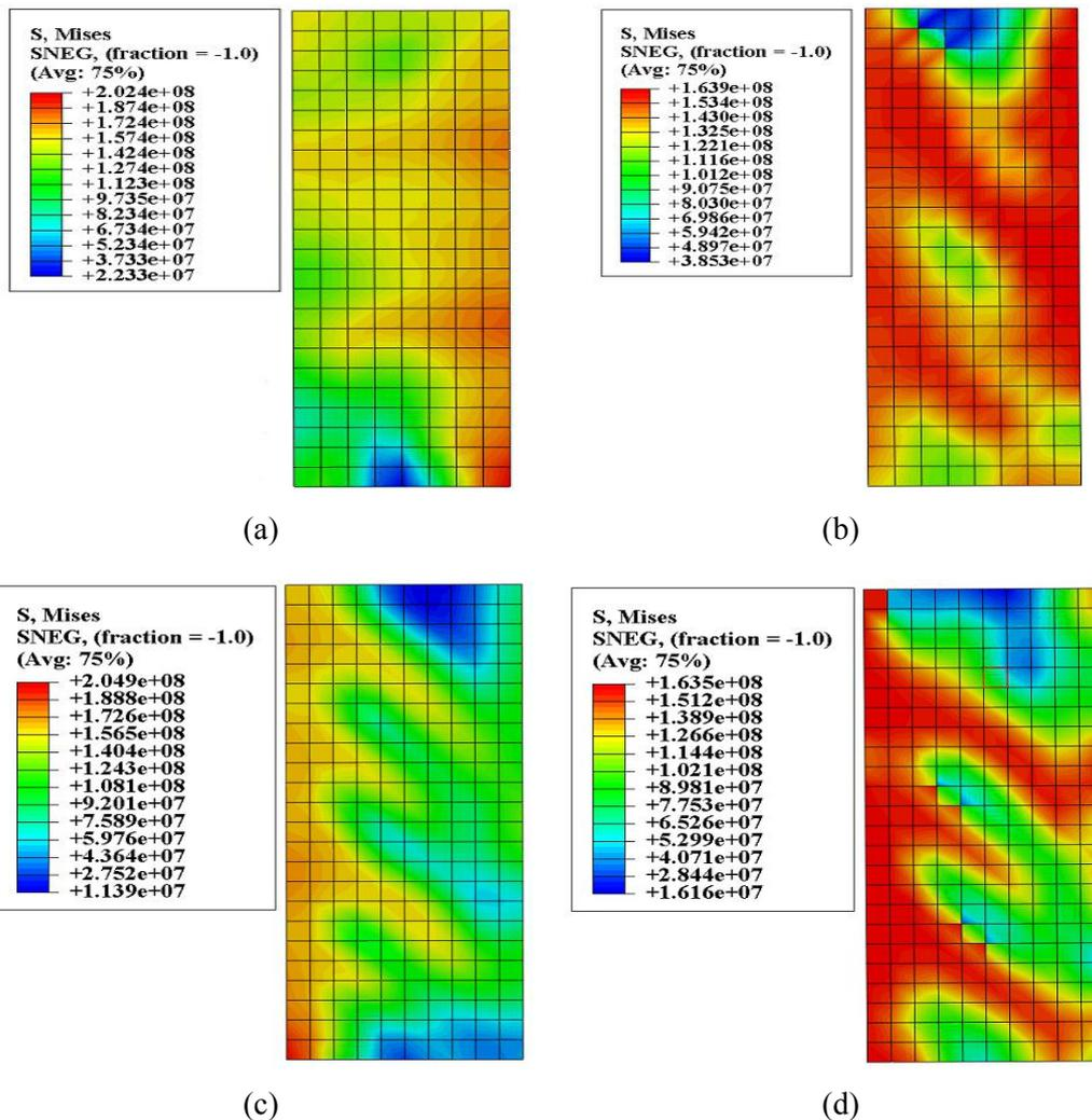
Fig.3 – Stress distribution of the EDMSPs: (a) bottom plate (longitudinal); (b) top plate (longitudinal); (c) bottom plate (transverse); (d) top plate (transverse)
