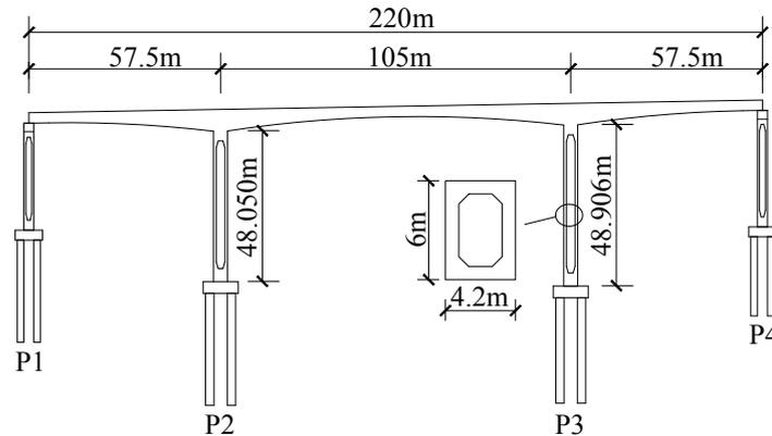
Fig.2 –Layout of the prototype bridge
