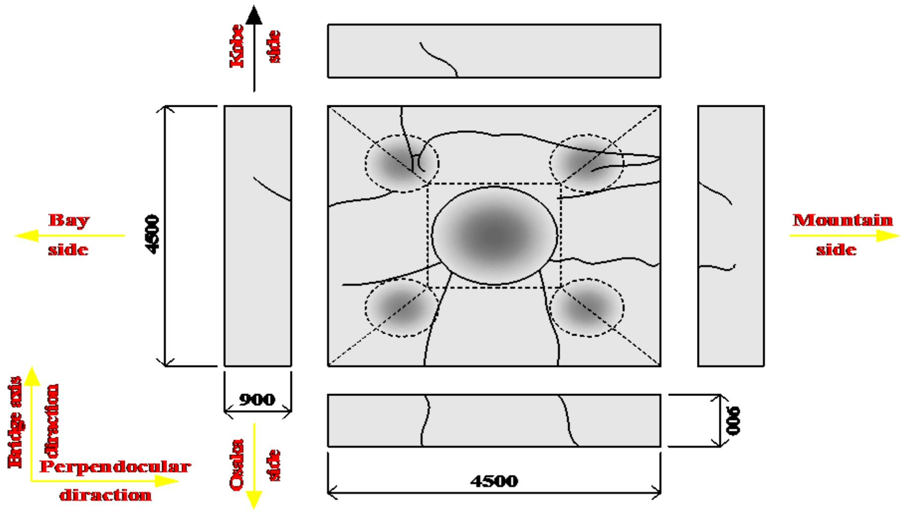
6. (8) Fig. Cracks observed on the footing
