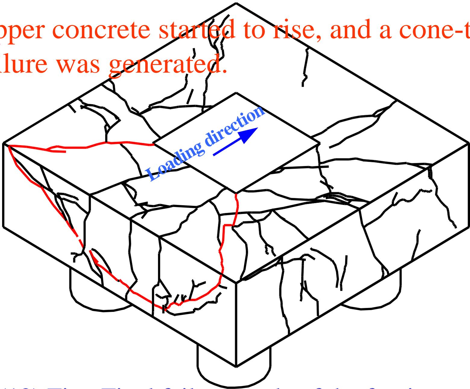
6. (12) Fig. Final failure mode of the footing
